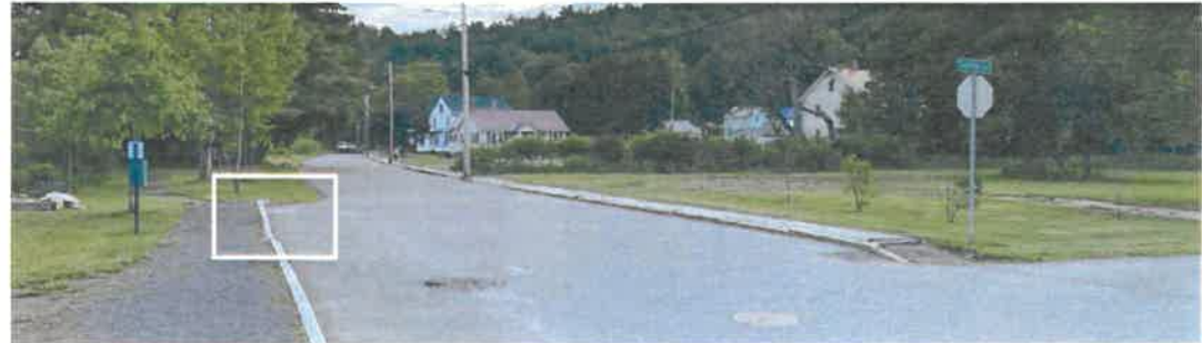
The parking area at Dog River Park is unpaved, making it difficult to navigate for some users, and has only one curb cut. This design paves the parking landing area for increased accessibility, and adds a second curb cut on the north end of the parking area.
