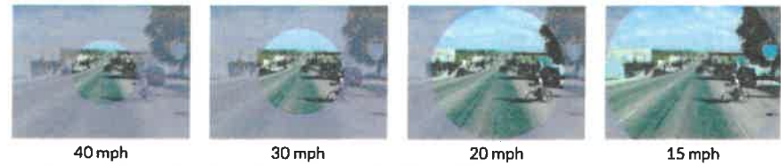
Graphic representing a driver's view of the road, which varies with speed (Source: Complete Streets; A Guide for Vermont Communities p. 15)
