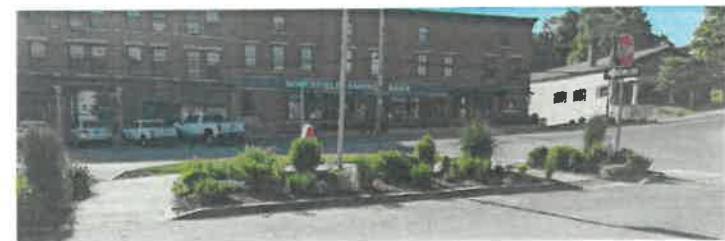
Image above: to provide a resting place for pedestrians while they cross wide the wide driveway entrance east of Napa Auto Parts, a pedestrian refuge island is proposed, similar to one found on the east side of Depot Square (pictured below)
